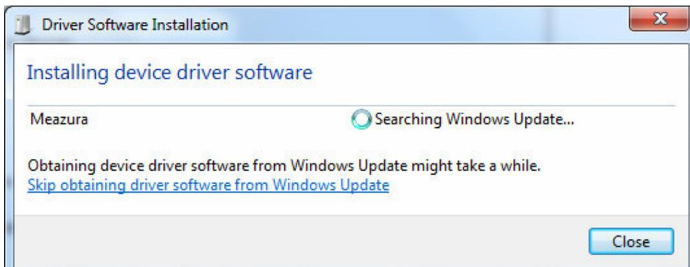
Windows is searching for the appropriate driver using 'Windows Update', which is the default behavior for a typical Windows 7 installation. However this process will fail because ACEECA has proprietary OEM drivers that aren't recognized by 'Windows Update'. You will instead see this dialogue and error bubble:
